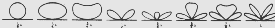
Fig. 4—Vertical patterns of resonant dipole for various heights above perfectly conducting ground.
